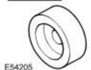
Remover rear differential rear bush 502-009/2
